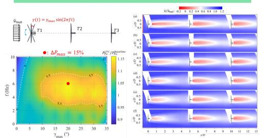
Wind tunnel experiments: a new cyclic yaw control (CYC) strategy has been investigated in a wind farm model in the EPFL atmospheric boundary layer wind tunnel. The results show that by applying CYC the power production can be improved up to 15%, compared to the baseline case. PIV measurements also reveal faster wake recovery for all individual wind turbines.
