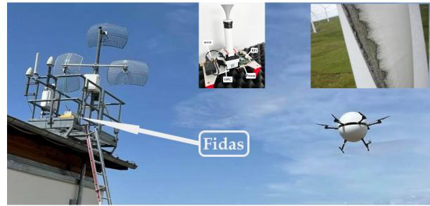
**Measuring aerosol particles** (e.g. sea spray) within a wind farm using multicopter-born Optical Particle Counter. The OPC arrangement includes a dryer to remove humidity from the particles. It compares well to a high-end fixed mounted Optical Aerosol Spectrometer, for PM1, PM2.5 and PM10 particle sizes. Can be used to determine leading edge erosion.
