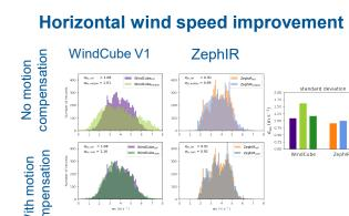
Floating Lidars: We have investigated the error induced by motion on shipbased lidars measurements and have applied motion compensation algorithms to remove these errors.
